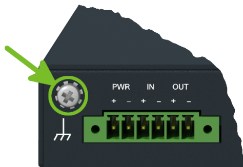
Figure 15: Position of the Grounding Screw
