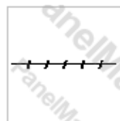
Pneumatic signal (long)
