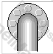
Flange with pipe extending down
