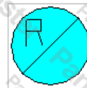
Duct elbow turning toward - return duct 2
